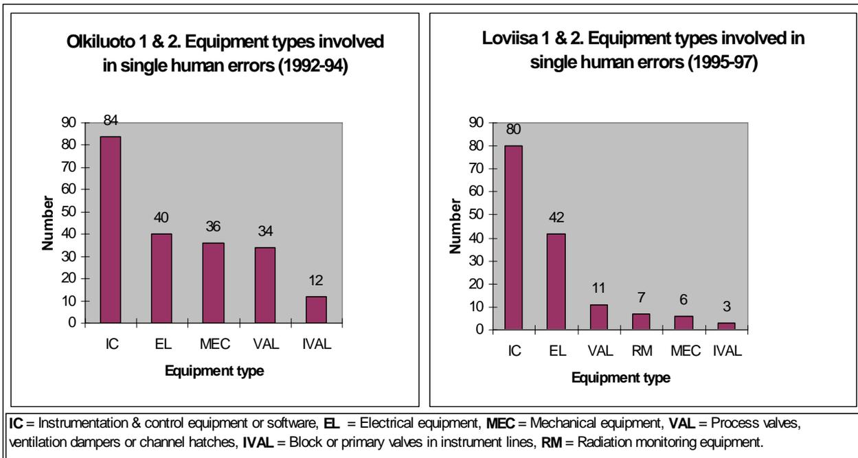
**Figure 4: Type of equipment affected by single human failures registered at Olkiluoto and Loviisa**
