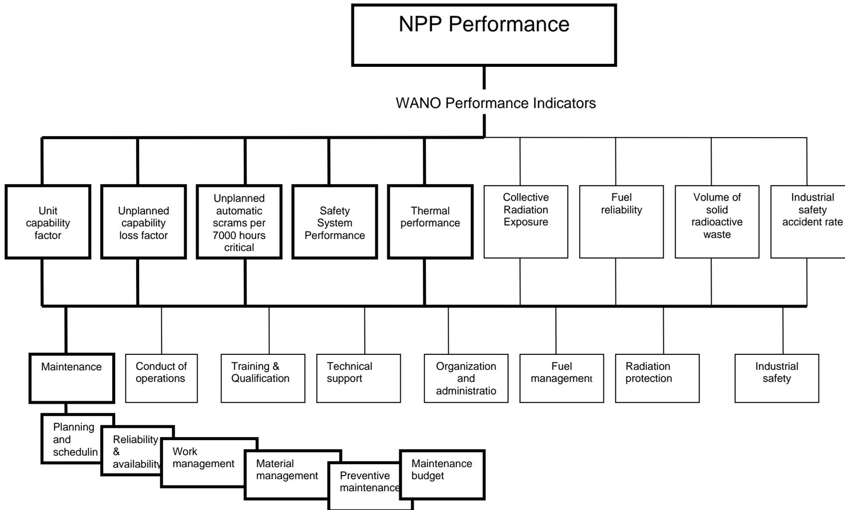
**Figure 1 Contribution of operational management programmes into the NPP performance**
