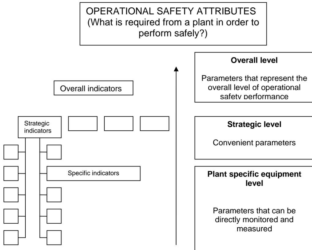
**Figure 2 IAEA approach to monitoring NPP operational safety performance.**
