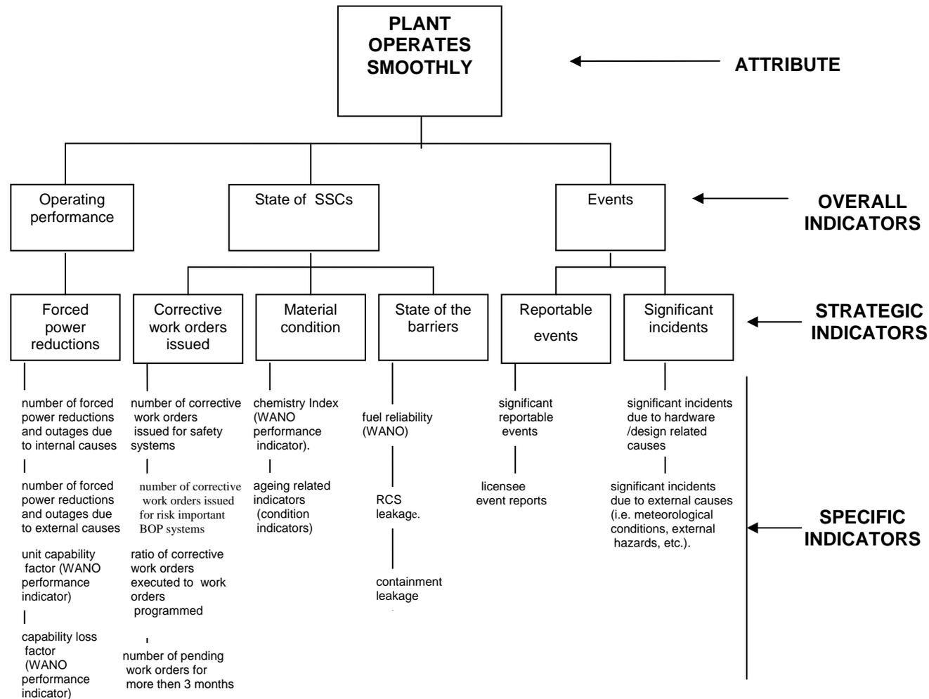
**Figure 4 Hierarchical structure of performance indicators for the operational attribute 'Plant operates smoothly'**
